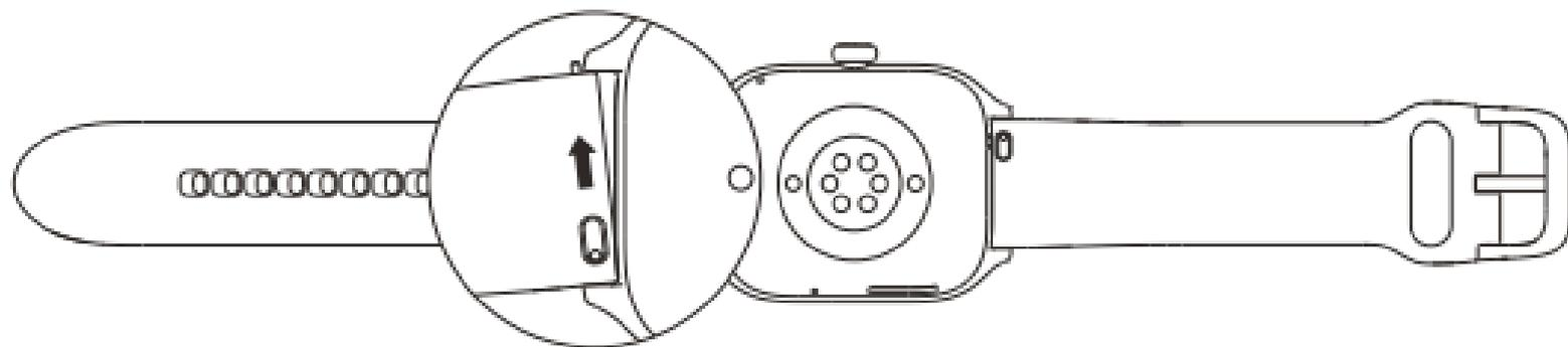
Note: Once the strap is assembled, pull the strap properly to ensure it is installed successfully.
