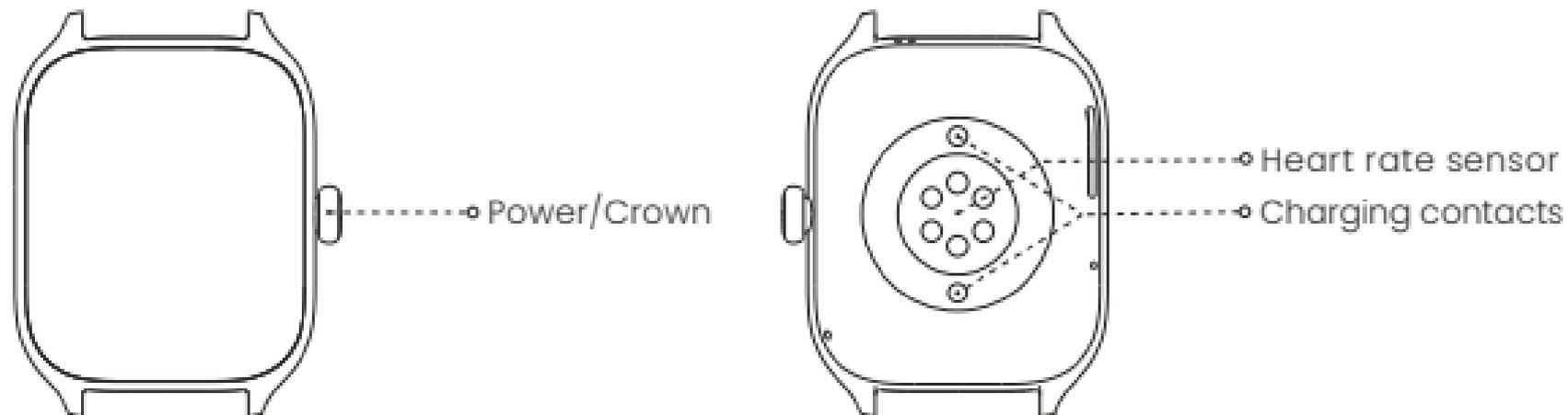
Note: Press and hold the power button to turn on the watch. If the watch cannot be turned on, please charge it and then try again.
